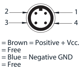
Connection M12x1 connector
